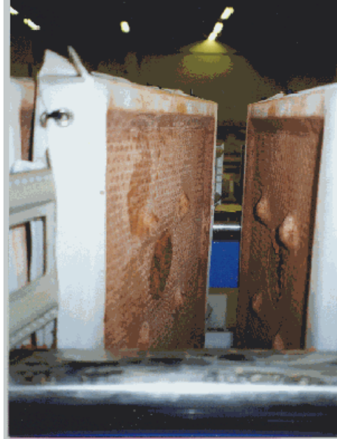
Figure 5: Filter chamber after discharging filtercake, showing very little solid adhering to the filter cloth.
