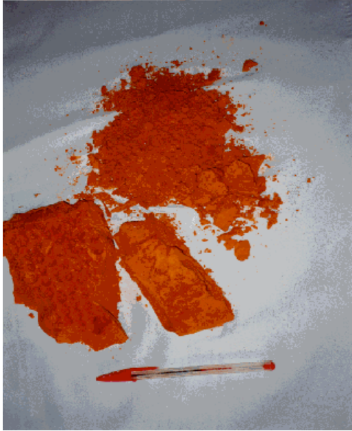
Figure 4: "Dry" filter cake arising from the filtration of hydrated ferric oxide.
